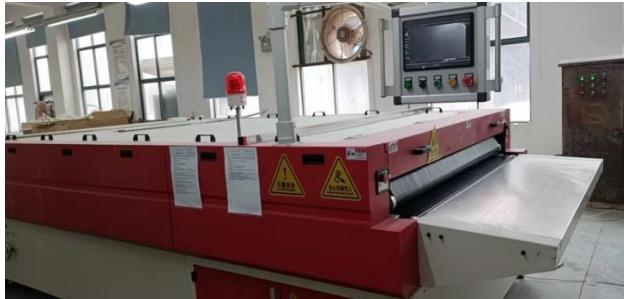
气凝胶隔热膜/隔热片涂布线
